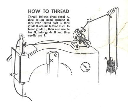
See that the machine is threaded properly, as improper threading causes breakage. The thread should feed firmly, but without pull or interruption.
